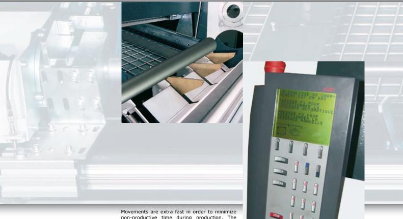
non-productive time during production. The magazine is equipped with a device that allows soft and quiet loading. The rollers keep friction to a minimum, regardless of the material or quality of the bars.
